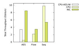
Figure 10: Throughput of AES encryption, flow classification, and network sequencer running on one CPU core and the LiquidIO NIC. 'CPU-AES-NI' uses AES-NI.
