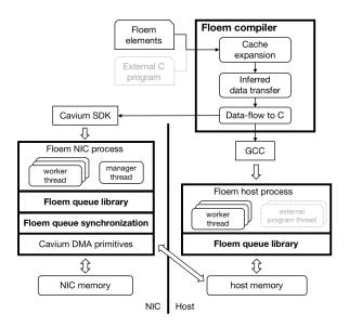
Figure 4: FLOEM system architecture
