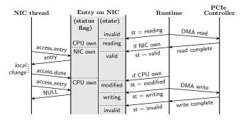
Figure 7: Transitions of a queue entry's status by a NIC worker thread and a NIC runtime manager thread
