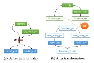
Figure 5: The key-value store's data-flow subgraph in the proximity of queue Q1 from the split CPU-NIC version
