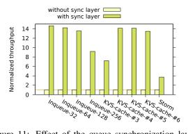
Figure 11: Effect of the queue synchronization layer. Throughput is normalized to that without the sync layer.
