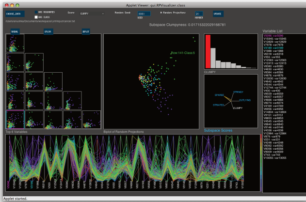
Figure 9: The Cancer dataset has over 16,000 dimensions and 14 classes or types of cancer. We maximize the Clumpy score and select a scatterplot in the SPLOM showing good separation of the purple class.
