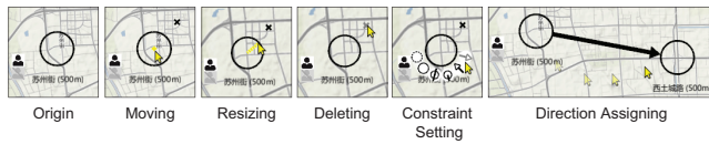
Figure 3: Interactions on Circular Filter: different functions are invoked by hovering on corresponding regions. Direction between filters is assigned by dragging from one to another.
